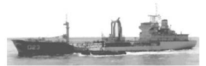
Type Number in Country Complement Capability Armament Speed Displacement LOA/Beam/Draft m(ft) Radar Replenishment Tanker 1 121 (13 officers) Carries 500 tons liquid cargo; 200 tons dry 2 x12.7-mm MGs 20 knots; Range: 9,000 miles at 15 knots 10,320 tons, full 135 x 19 x 7.5 (442.9 x 62.3 x 24.6) DF LOOP
