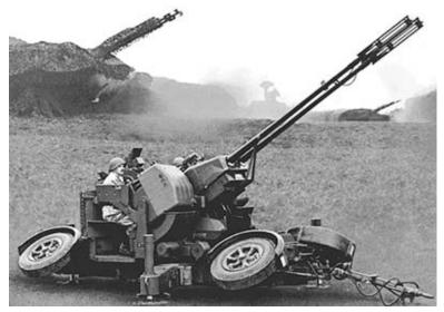
Crew Tactical Range Maximum Ranges Rate of Fire (Per Barrel) Emplacement Time Combat Weight 3 (1 for GDF-005) 4,000 m 8,500 m (vertical), 11,200 m (horizontal) 550 rd/min 2 to 4 min 6,300 - 6,400 kg
