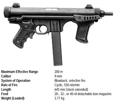
**NOTE:** Weapon has two safety systems: a grip safety in the front of the pistol grip, below the trigger must be held in before the action can be cocked; a push-button safety above the pistol grip locks the grip safety until pushed to the right.
