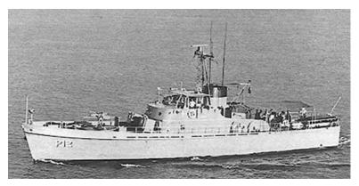
Role Complement Speed Displacement LOA/Beam/Draft m(ft) Guns Radar Sonar Coastal patrol 15 19.6 knots 103.8 tons (full) 29 x 6.2 x 2 (95 x 20.3 x 6.6) 7 x 12.7-mm/90 MG, 1 x 81-mm mortar combination Raytheon-2840 QCU-1
