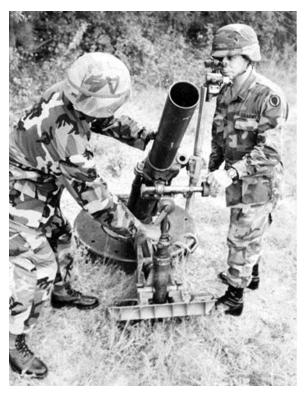
Crew Caliber Rate of Fire Maximum Range Tube Length Weight Ammunition 2 107-mm 18 rds/min max; 3 rds/min sustained 5,650 m (with tactical CS XM630) 1.524 m 305 kg Fires HE, Smoke, Illumination, Gas and Tactical CS
