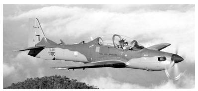
Role Light attack /trainer plane Crew 2 (in tandem) 2 x 12.7-mm guns; assorted cannon, bombs, and air-to-air missiles Armament Wing Span 11.14 m Length 11.42 m Weight (Empty) 2,420 kg Max Level Speed 557 km/h Range 1,568 km
