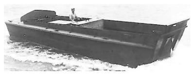
Role Complement Speed Displacement LOA/Beam/Draft m(ft) Vehicle/personnel landing 5 10 knots 12.1 tons (full) 10.9 x 3.4 x 1.1 (35.8 x 11.2 x 3.6)
