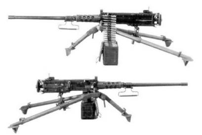
Maximum Effective Range Caliber System of Operation Overall Length Feed Weight (Loaded) 1,500 m 12.7- x 99-mm Short recoil 1.651 m 100-rd disintegrating link belt 38 kg
