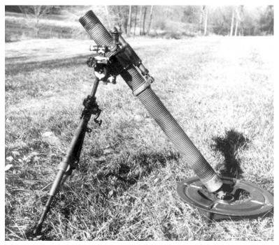
Crew Feed Length of Barrel Elevation 2 Muzzle loaded 1.295 m 800-1,500 mils
