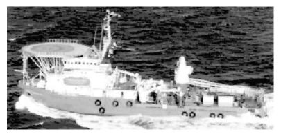
Role Complement Speed Displacement (tons) LOA/Beam/Draft m(ft) Submarine rescue 65 14.5 knots 3,030 (full) 78.2 x 17.5 x 4.7 (256.6 x 57.4 x 15.2)
