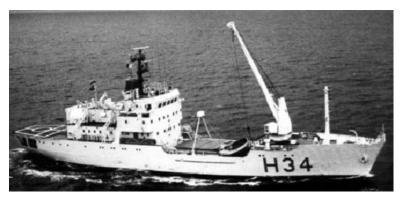
Type Complement Speed Displacement LOA/Beam/Draft m(ft) Radar Sonar Aircraft Bouy Tender 80 13 knots 2,390 tons (full) 75.6 x 13 x 3.7 (248 x 42.7 x 12.1) 2 DECCA Series ECHO SOUNDER, 1 OMEGA Bell 206B
