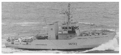
Type Complement Speed Displacement LOA/Beam/Draft m(ft) Buoy tender 19 (2 officers) 14 knots 890 tons (full) 54.5 x 7.5 x 1.8 (178.8 x 24.5 x 6)
