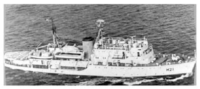
Role Complement Aircraft Speed Displacement LOA/Beam/Draft m(ft) Radar Sonar Hydrographic survey 102 Can support one Bell JetRanger or UH-12 15.7 knots 1,916 tons (full) 77.9 x 12 x 3.9 (255.6 x 29.4 x 12.8) Navigation: Racal DECCA TME 1226C; I-band MS 26
