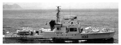
Role Complement Speed Displacement LOA/Beam/Draft m(ft) Radar Sonar Hydrographic survey 34 15 knots 350 tons (full) 44.7 x 6.5 x 2.8 (146.7 x 21.3 x 9.2)' DECCA-1226 ECHO SOUNDER
