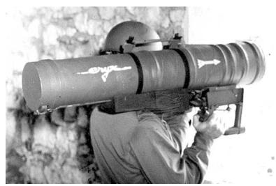
Role Maximum Effective Range Caliber Length Armor Penetration Emplacement Time Short Range Anti-Tank Missile 600 m 136-mm 905 mm 900 mm 5 seconds
