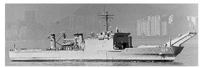
Role Complement Speed Displacement LOA/Beam/Draft m(ft) Guns Radar Sonar Tank landing 187 22 knots 8,450 tons (full) 159.2 x 21.2 x 5.3 (522.3 x 69.6 x 17.4) 2 x twin 76-mm/50, 1 x Gatling 20-mm/70 AN/SPS-67, LN-66 ECHO SOUNDER
