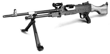
Maximum Effective Range Caliber System of Operation Length Feed Device Weight (Loaded) 1,500 m 7.62 x 51-mm Gas, automatic 1.26 m Belt 13.92 kg (with butt stock and bipod)
