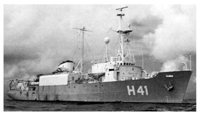
Role Complement Speed Displacement LOA/Beam/Draft m(ft) Oceanographic research 40 13.5 knots 1,432 tons (full) 63.5 x 12 x 5.9 (208.3 x 39.4 x 19.4)
